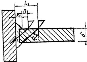
$$\delta = 10 - 20 \text{ мм} \quad \alpha_1 = 65^\circ \pm 2^\circ, \\ L_1 = K_1 + 2,15\delta;$$
